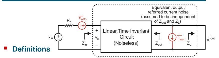
Noise Factor  $= F = \frac{SNR_{in}}{SNR_{out}}$
