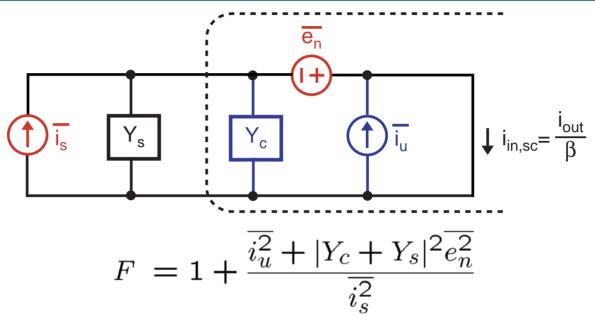
We can replace voltage and current noise currents with impedances and admittances
