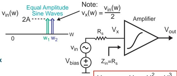
IIP3 referenced to V<sub>x</sub> (rms voltage)
