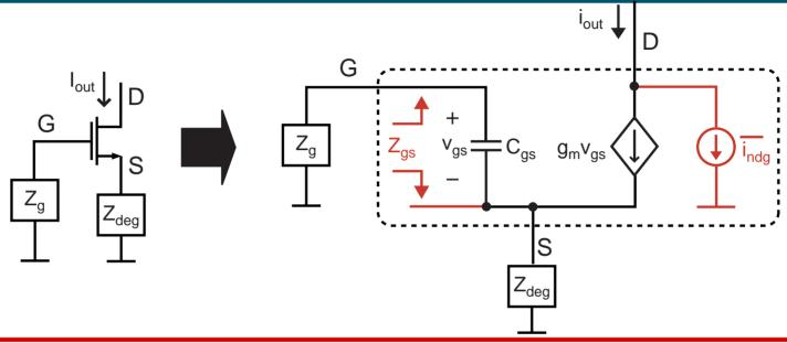
$$\frac{\overline{i_{ndg}^2}}{\Delta f} = \frac{\overline{i_{nd}^2}}{\Delta f} \left( |\eta|^2 + 2Re \left\{ c\chi_d \eta^* Z_{gsw} \right\} + \chi_d^2 |Z_{gsw}|^2 \right)$$
