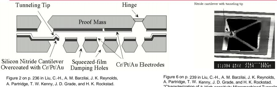
"Characterization of a High-sensitivity Micromachined Tunneling Accelerometer with Micro-g Resolution." *Journal of Microelectromechanical Systems* 7, no. 2 (June 1998): 235-244. © 1998 IEEE. A. Partridge, T. W. Kenny, J. D. Grade, and H. K. Rockstad. "Characterization of a High-sensitivity Micromachined Tunneling Accelerometer with Micro-g Resolution." *Journal of Microelectromechanical Systems* 7, no. 2 (June 1998): 235-244. © 1998 IEEE.
