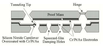
Figure 2 on p. 236 in Liu, C.-H., A. M. Barzilai, J. K. Reynolds, A. Partridge, T. W. Kenny, J. D. Grade, and H. K. Rockstad. "Characterization of a High-sensitivity Micromachined Tunneling Accelerometer with Micro-g Resolution." *Journal of Microelectromechanical Systems* 7, no. 2 (June 1998): 235-244.
