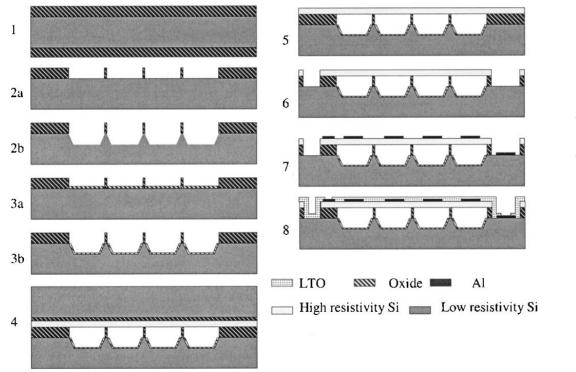
Figure 1 on p. 130 in Huang, Y., A. S. Ergun, E. Haeggstrom, M. H. Badi, and B. T. Khuri-Yakub. "Fabricating Capacitive Micromachined Ultrasonic Transducers with Wafer-bonding Technology." *Journal of Microelectromechanical Systems* 12, no. 2 (April 2003): 128-137. © 2003 IEEE.
