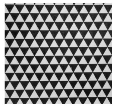
The above is a photograph of a portion of a flat target used for camera calibration as well as estimation of camera distortions.
