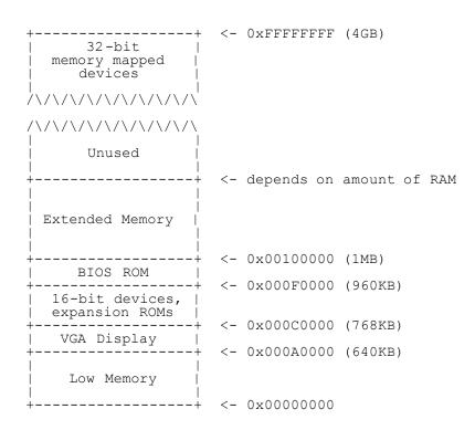
The first PCs, which were based on the 16-bit Intel 8088 processor, were only capable of addressing 1MB of physical memory. The physical address space of an early PC would therefore start at 0x00000000 but end at 0x000FFFF instead of 0xFFFFFFFF. The 640KB area marked "Low Memory" was the *only* random-access memory (RAM) that an early PC could use; in fact the very earliest PCs only could be configured with 16KB, 32KB, or 64KB of RAM!
