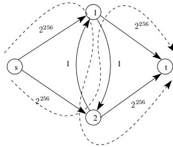
Figure 6.7: An example for which the Ford-Fulkerson, in the stated form, might perform very badly. The algorithm runs slowly if at each step, the augmentation path is either  $s \rightarrow 1 \rightarrow 2 \rightarrow t$  or  $s \rightarrow 2 \rightarrow 1 \rightarrow t$  (shown with dashed lines). At an augmentation, the flow will increase by at most 2.
