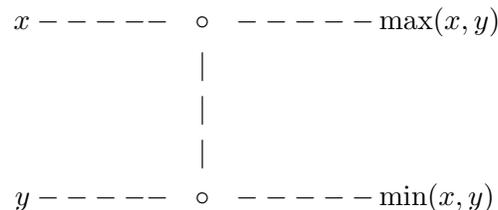
Such a network of comparators is a valid sorting network if for any possible set of values on the  $n$  input wires, the values on the  $n$  output wires are in sorted order. There exist sorting networks with  $n \log^2 n$  comparators. More efficient sorting networks also exist, but are very complex.
