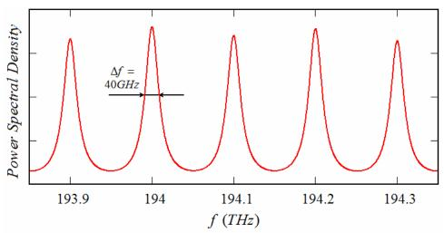
At the output of the fiber, each of these channels must be separated from the others before information carried by this channel can be used. Suppose we want to use a Fabry-Perot resonator as a filter to select the single channel at 194 THz. The two mirrors of the Fabry-Perot are identical and are separated by material with a refractive index of n = 1.5.
