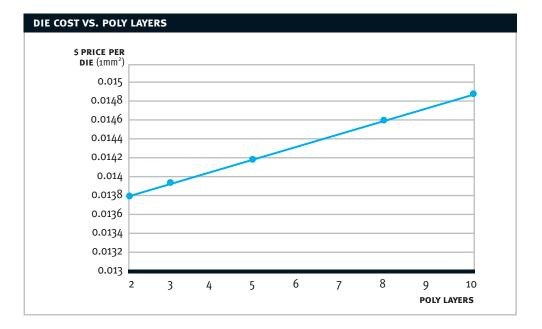
Figure 13: Poly Layers Vs. Die Cost (25 Mask, 5 Metal).
