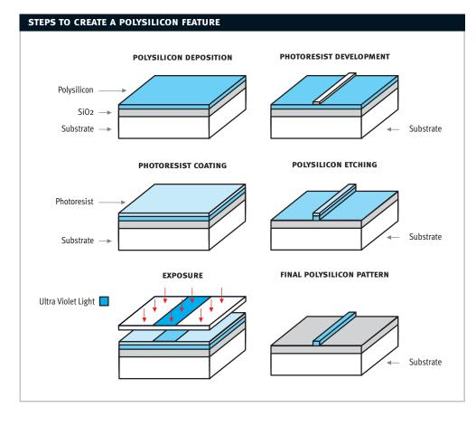
The following steps are repeated in the appropriate process sequence until the silicon die is ready:
