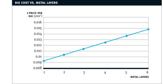
Figure 14: Metal Layers Vs. Die Cost (2 Poly, 25 Mask).
