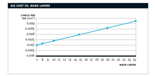
Figure 12: # Mask Layers Vs. Die Cost (1 Metal, 1 Poly)
