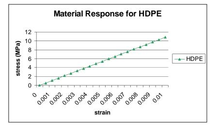
One can observe that the plots for all three materials produce straight lines with the slope being equal to the Young's Modulus of the material. The plot for HDPE was reproduced on a second graph to make the stress values readable.
