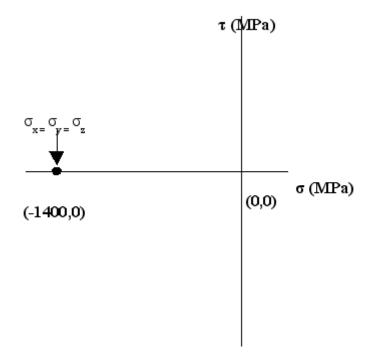
As all of the shear forces are equal to zero, we see that we are already in the principal stress state with each of the principal normal stress being equal to - 1400MPa. The principal axes are the x-, y-, and z-axes as noted in our original diagram and no rotation is necessary.
