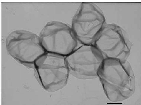
PEM hollow microcapsules built on PS microsphere templates subsequently dissolved. (Rubner & coworkers, MIT)
