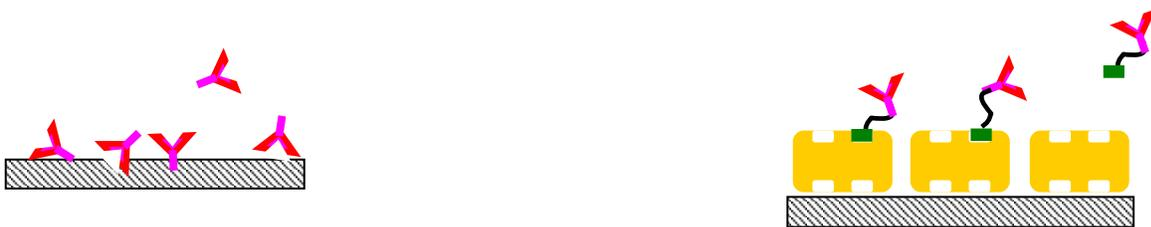
**Covalent binding** (via  $-\text{COOH}$ ,  $-\text{NH}_2$ ,  $-\text{OH}$  chemistries) or crosslinking (ex., via glutaraldehyde) to transducer or membrane surface
