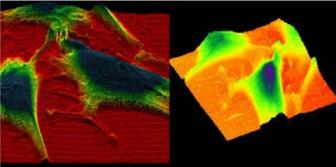
Height image of **endothelial cells** taking in fluid using Contact Mode AFM. 65 µm scan courtesy J. Struckmeier, S. Hohlbauch, P. Fowler, Digital Intruments/Veeco Metrology, Santa Barbara, USA.
