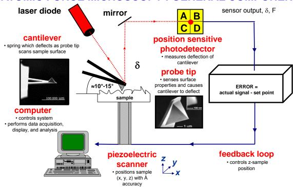
**Advantages**: 1) Unlike electron microscopes, samples do not need to be coated or stained, minimal damage, 2) Unlike electron microscopes, samples can be imaged in fluid environments (near-physiological conditions), 3) Unlike STM samples do not need to be conductive, 4) Sub-nm resolutions have been achieved on biological samples (detailed information on the molecular conformation, spatial arrangement, structural dimensions, rate dependent processes, etc.)
