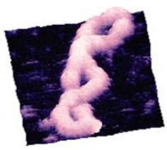
The high resolution of the SPM is able to discern very subtle features such as these two linear dsDNA molecules overlapping each other. 155nm scan.
