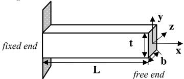
**Figure 1.** Nomenclature for a cantilevered beam with rectangular cross section ; L=length or span (m), b=width (m), t=height or thickness (m), I=moment of inertia of cross-sectional area (m<sup>4</sup>), E=Young's (elastic) modulus (Pa=N/m<sup>2</sup>), and EI=flexural modulus (Nm<sup>2</sup>)
