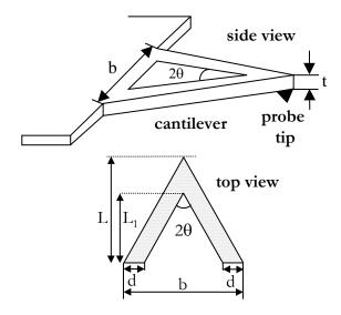
Figure 6. Dimensions of a V-shaped cantilever beam
