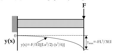
Figure 4. Elastic curve of cantilevered beam
