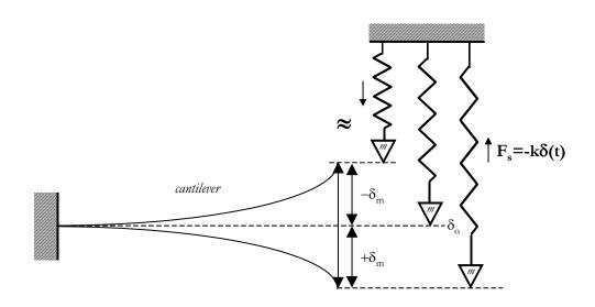
Figure 7. Thermal oscillation of a free cantilever beam
