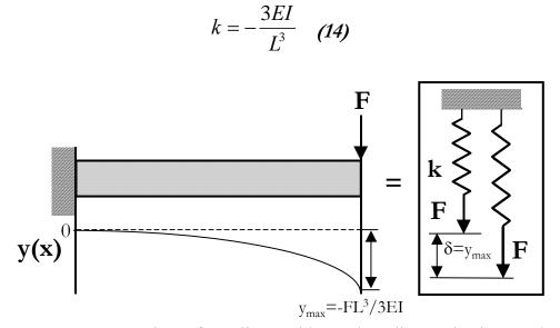
**Figure 5.** Representation of cantilevered beam by a linear elastic, Hookean spring
