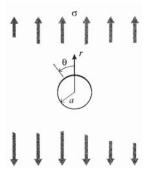
Figure 2: Circular hole in a uniaxially stressed plate
