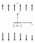
Figure 6: Sharp crack in an infinite sheet.
