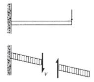
Figure 8: Shearing displacements in beam bending.
