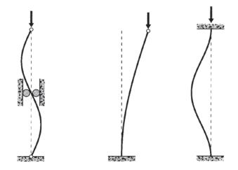
Figure 7: Effect of lateral support and end conditions on beam buckling.
