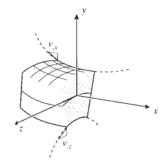
Figure 5: Anticlastic curvature.
