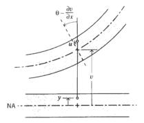
Figure 1: Geometry of beam bending.
