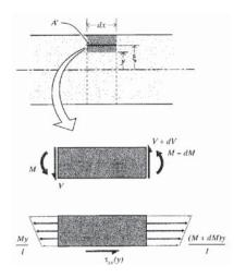
Figure 9: Shear and bending moment in a differential length of beam.
