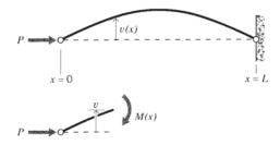
Figure 6: Imminent buckling in a beam.
