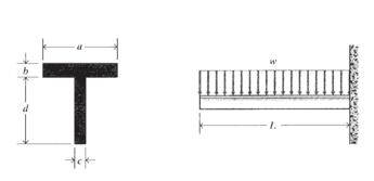
Figure 4: A cantilevered T-beam.
