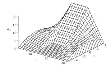
Figure 14: Variation of principal stress  $\sigma_{p1}$  in four-point bending.
