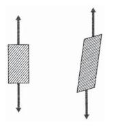
Figure 4: Shear-normal coupling.
