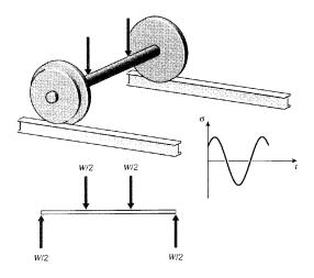
Figure 3: Fatigue in a railcar axle.
