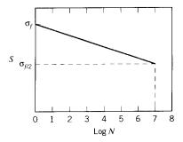
Figure 9: Linear S-N curve.
