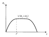
Figure 10: Transverse stress at crack tip.
