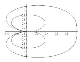
Figure 11: Normalized plastic zone shapes for plane strain (inner contour) and plane stress (outer contour).
