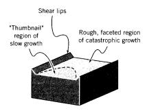
Figure 12: Fracture surface topography.
