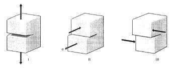
Figure 6: Fracture modes.
