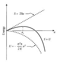
Figure 2: The fracture energy balance.
