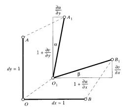
Figure 4: Finite displacements.
