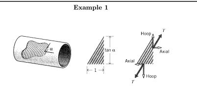
Figure 6: Filament-wound cylindrical pressure vessel.
