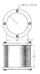
Figure 9: A bolt-clamped pressure vessel.
