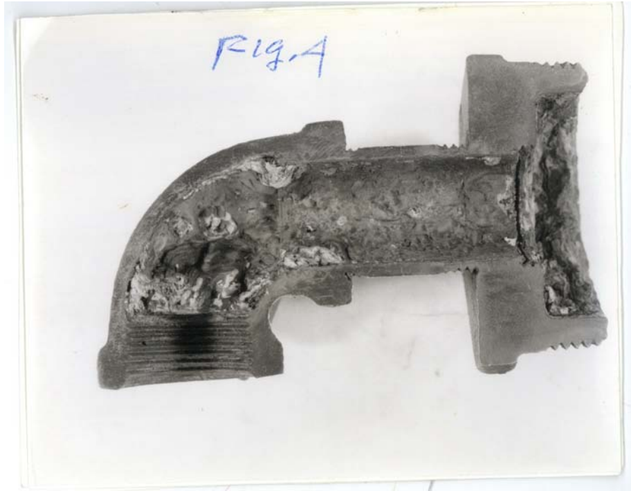
Figure 4: Sliced in half, the corroded bushing has been polished and etched.
