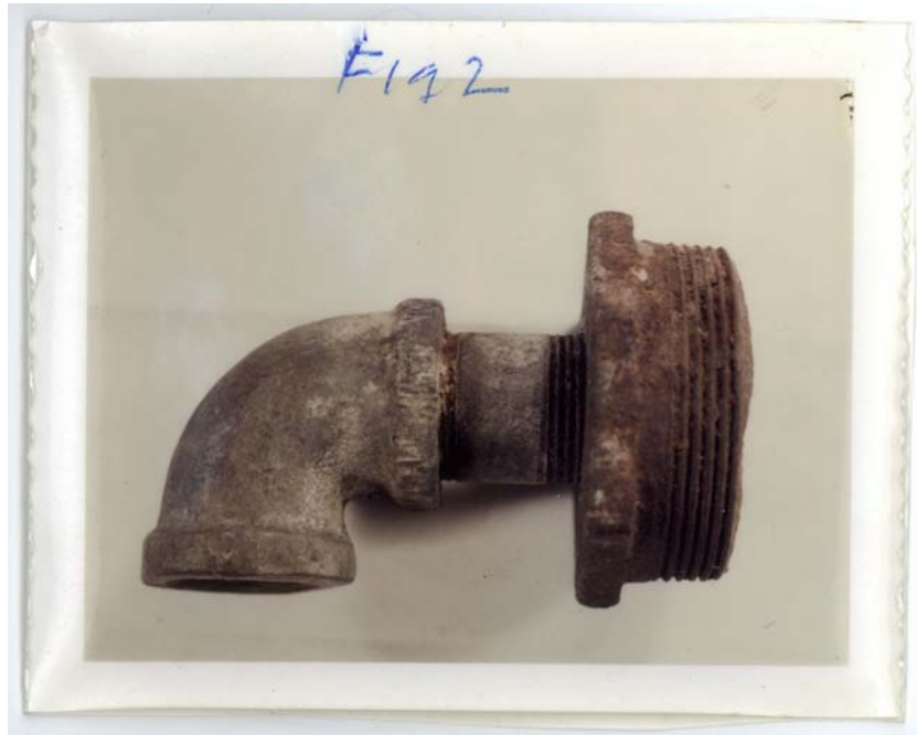
Figure 2: Failed bushing, showing corrosion.
