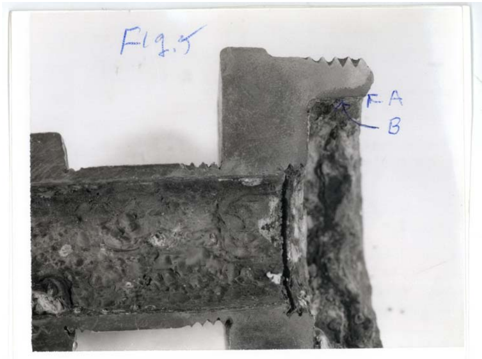
Figure 5: A closeup of the etched metal shows magnetite at the valve.
