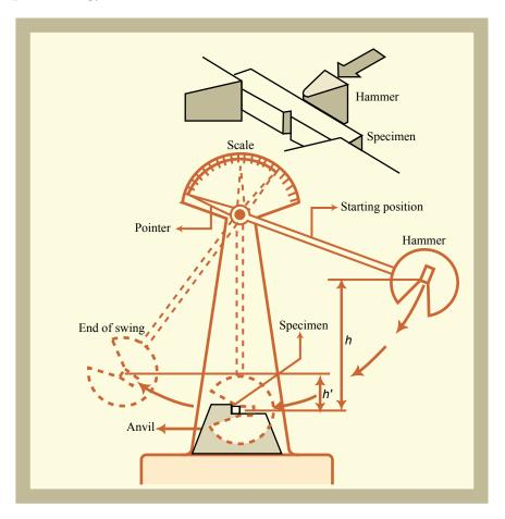
Geometry of Charpy impact test.
