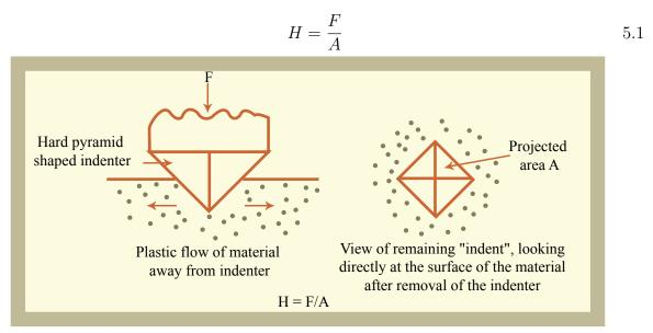
Figure 3: Schematic of a hardness test
