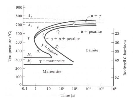
Figure 2: Time-Temperature-Transformation (TTT) curve for carbon steel AISI 1050.
