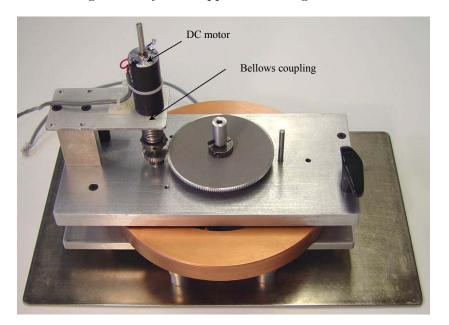
Figure 2: Flywheel apparatus with gear train and DC motor.
