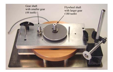
Figure 1: Flywheel apparatus with gear train.
