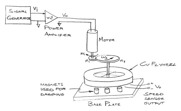
Figure 4: System configuration.
