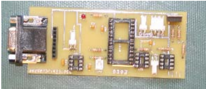
Image 6 – DB9, Molex, Voltage Regulator, and SIP installed
