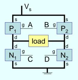
To make flow UL to LR, set A = GND and D =  $V_s$ To make flow UR to LL, Set B = GND and C =  $V_s$
