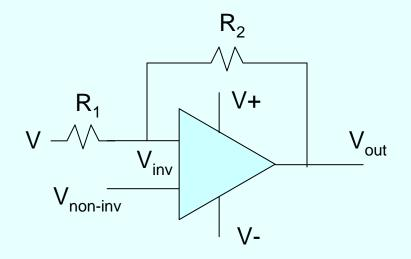
Voltage bias useful for bringing signal levels into the range of sensors.
