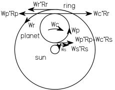
ref: Gear Drive Systems; Design and Application, P. Lynwander TJ184.L94 1983 N.B. in this development  $W_s$  and  $W_c$  are clockwise and  $W_r$  and  $W_p$  are ccw
