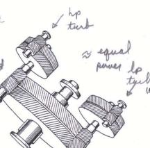
(f) Double reduction, single input, locked train gear elements of for 1/2 power > smaller but more part, torsional blex shaft required
