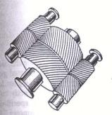
(d) Double reduction, double input, articulated tandem (in line) articulated - flex coupling between and a pinion
