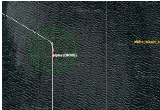
Figure 2: The Pulse Behavior: The behavior simply generates a range pulse after it observes that a waypoint has been achieved. The range pulse is a posting to the variable footnotesize RANGE_PULSE .
