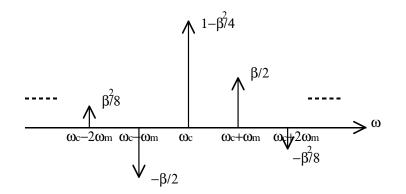
Figure 3: Spectrum for FM, with a modulating signal of a single sinusoid.
