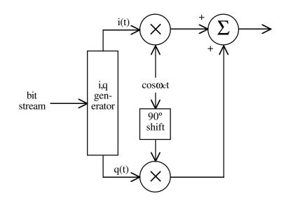
Figure 5: Digital quadrature modulator.
