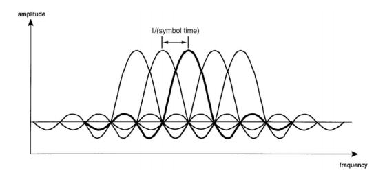
Figure 9: If COFDM signals are rectangular pulses in time, they are sinc-shaped in frequency. If the carriers are spaced orthogonally, there is no interference from one carrier to another. (Adapted from Maddocks, 1993)
