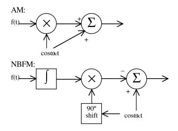
Figure 2: Modulators for AM and NBFM.
