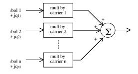
Figure 8: Orthogonal frequency-division multiplexing.
