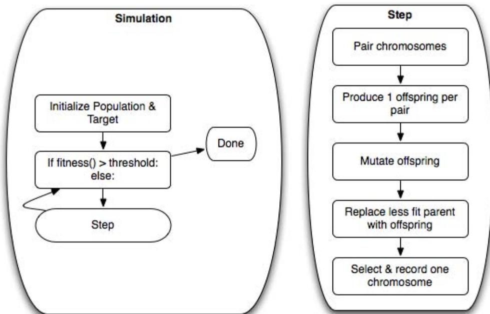
Figure 2 the control logic of Simulation and Step.
