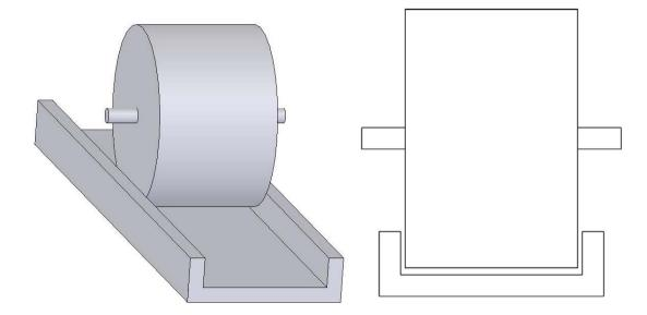
The simplest design is to have a regular caster in a groove, as shown below:
