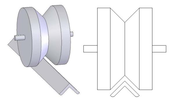
This will provide very accurate positioning, as the neutral position is a stable equilibrium, and the likelihood of undue friction or binding is small. However, it may be more likely to snag feet of actors as they walk over it, and it must also be attached properly to the stage. If the facilities and the material is available, attachment can be as simple as welding the L extrusion onto a long, thing plate, and then bolting the plate to the stage.
