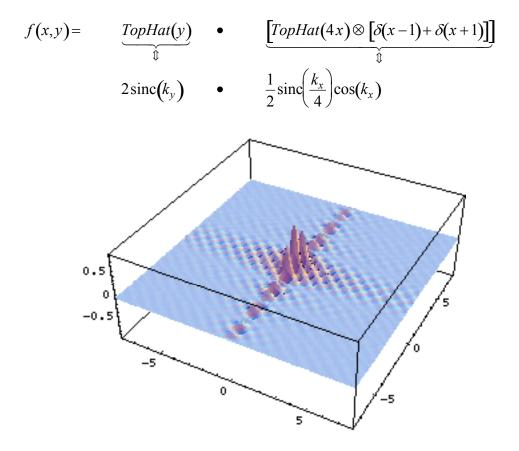
d. The Fourier Transform of the X-ray source has pronounced oscillations. To remove these oscillations one can file down the edges which replaces a sharp edge by a triangular edge:
