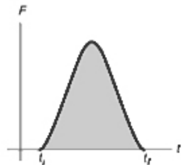
(A) A force acting on a particle may vary in time. The impulse is the area under the force versus time curve.
