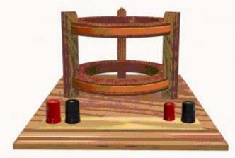
Figure 3 Helmholtz Coil Apparatus
