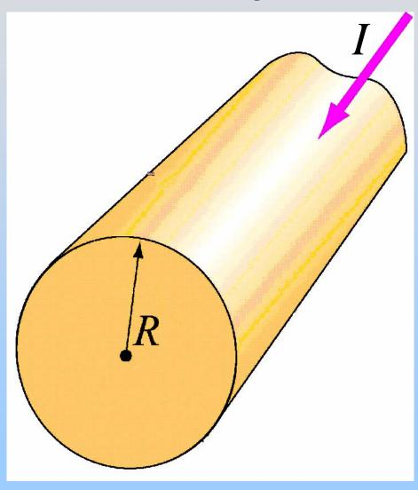
A cylindrical conductor has radius R and a non-uniform current density with total current:
