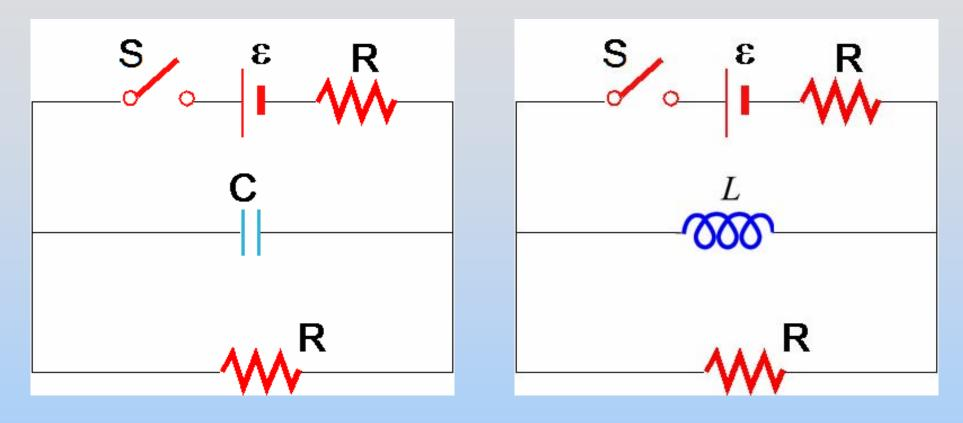
For the two above circuits sketch the currents through the two bottom branches as a function of time (switch closes at t = 0, opens at t = T). State values at  $t = 0^+$ ,  $T^-$ ,  $T^+$
