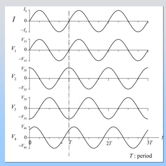
Consider an RLC circuit. You measure the voltage across all 4 elements (V<sub>1</sub>...) Which is which? Are we above or below resonance? What are R,L,C? What is  $\omega_0$ ?
