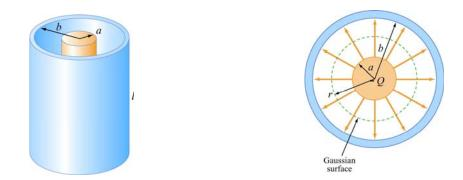
Two concentric cylinders have radii *a* and *b* and height *l*, with b > a. The inner cylinder carries total charge -*Q*, and the outer cylinder carries total charge *Q*. *We ignore end effects*.
