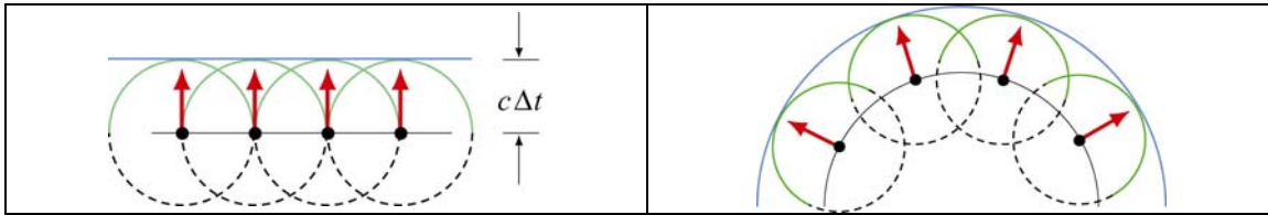
Figure 14.4.1 Propagation of wave based on Huygens’s principle.
