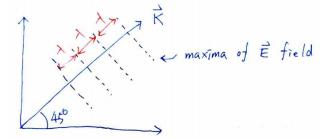
$$\vec{B} = \frac{1}{c}\hat{k} \times \vec{E} \; \Rightarrow \; \vec{B}(x, y, z) = \frac{E_0}{c}\hat{z}\cos\left(\frac{\sqrt{2}\pi}{\lambda}(x+y) - \omega t\right)$$
