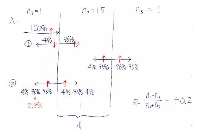
We are looking at the interference between 1 and 2. Question: what is the thickness d that is needed to have constructive interference? Phase difference: 1-2:
