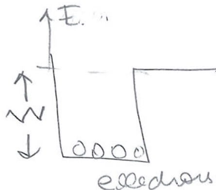
Figure 1: Electrons in a metal are bound. If the photon energy is greater than the work function W an electron may be ejected.
