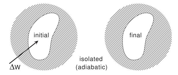
Final state is independent of <u>how</u>  $\Delta W$  is applied. Final state is independent of <u>which</u> adiabatic path is followed.
