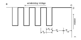
FIG. 4: Plot of anode current against accelerating voltage  $V_{cg}$  implied by set of idealized assumptions.
