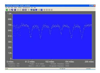
FIG. 7: Typical Mossbauer spectrum using an enriched Fe-57 foil acquired by the Spectech UCS-20 multi-channel analyzer. Distance between Co-57 and proportional counter detector window is  $\sim \! 10 \, \mathrm{cm}$ . Integration time = 3000 passes  $\sim \! 10 \, \mathrm{min}$ utes. Co-57 had  $\sim \! 5 \, \mathrm{mCi}$  of activity.
