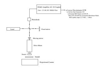
FIG. 8: Schematic diagram of the Michelson interferometer for calibration of the velocity sweep. Be particularly sensitive to try and block any stray reflections of the HeNe laser from interferometer into another another portion of the lab. Block as necessary using black posterboard or index cards.
