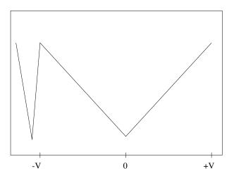
FIG. 9: Ideal appearance of the multichannel scaler screen after several minutes of operation with the interferometer velocity calibrator. The sharp feature at the start is produced during the rapid reversal of the velocity of the piston at the high speed end of its stroke. In reality, the bottom of the "V" will probably be truncated due to the low amplitude of the pulses during the low-velocity portion of the sweep.
