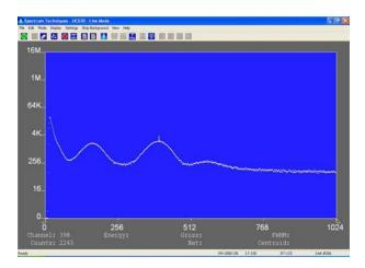
FIG. 6: Typical Co-57 pulse height spectrum acquired by the Spectech UCS-20 multi-channel analyzer. Distance between Co-57 and proportional counter detector window is  $\sim$ 10cm. Integration time = 100s. Co-57 had  $\sim$ 5mCi of activity.
