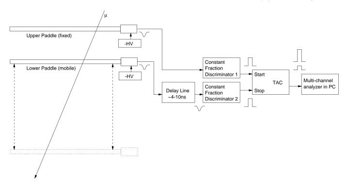
FIG. 2: (a) Arrangement for measuring the speed of cosmic-ray muons.
