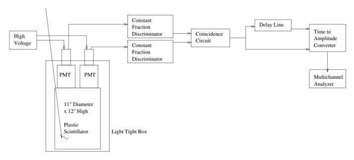
FIG. 4: Arrangement for measuring the mean life of muons
