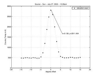
FIG. 6: Sun Scan Elevation
