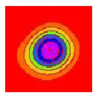
FIG. 5: Typical result from an "npoint" measurement of the Sun's brightness temperature. The countour plot is generated from a 5x5 series of measurements spaced by 1/2 the antenna beamwidth as specified in the srt.cat text file within the CassiSRT folder on the hard drive.
