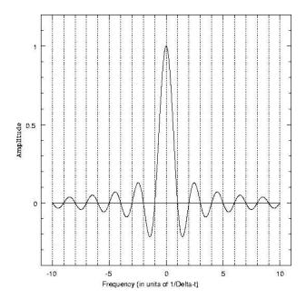
FIG. 16: The Fourier transform of a uniform window of width  $\Delta t$ . The vertical dotted lines show the centers of the frequency channels in the sampled power spectrum, assuming the spectral line is exactly at the center of one channel (which it may not be).
