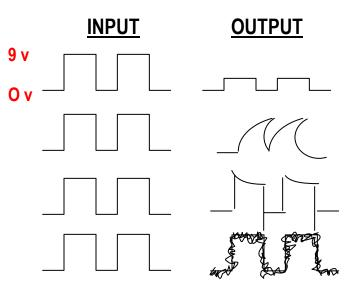
DISTORTION = CAUSED BY CAPACITANCE, INDUCTANCE, RESISTANCE (SYSTEMATIC)
