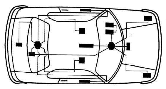
Topography of vehicle multi-plex system with central control, modules for the instrument readings, lights, doors, seats, centre console and central rear light unit.
